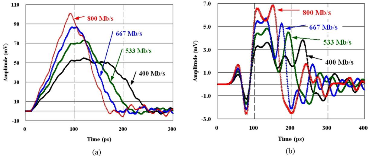
Fig. 12. Voltage waveforms of crosstalk for different pulse speeds. (a) NEXT. (b) FEXT. (Color version available online at <http://ieeexplore.ieee.org>.)
