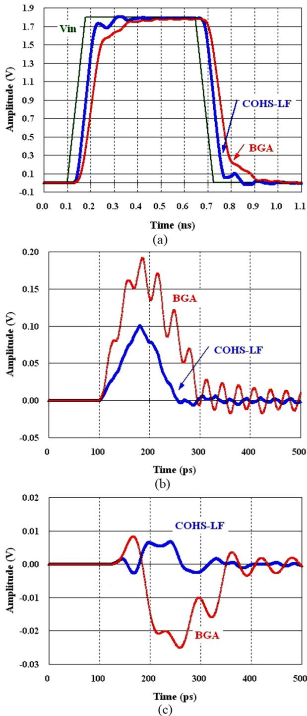
Fig. 11. Transient analyses for COHS-LF and BGA packages. (a) Input ( $V_{in}$ ) and output waveforms of Lead 7 (COHS-LF package) and DQ3 (BGA package). (b) Near-end crosstalk of Lead 8 (COHS-LF package) and DQ4 (BGA package). (c) Far-end crosstalk of Lead 8 (COHS-LF package) and DQ4 (BGA package). (Color version available online at <http://ieeexplore.ieee.org>.)
