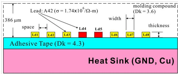
Fig. 3. Cross section of COHS-LF package for 50- $\Omega$  impedance per lead. (Color version available online at <http://ieeexplore.ieee.org>.)
