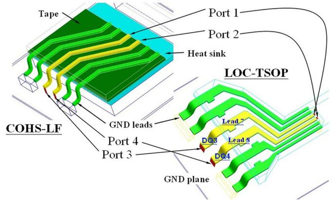
Fig. 5. 3-D structures for COHS-LF and LOC-TSOP packages. (Color version available online at <http://ieeexplore.ieee.org>.)
