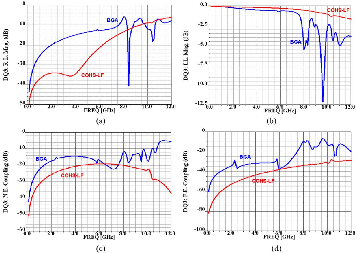
Fig. 8. Comparison of  $S$ -parameter in magnitude between the COHS-LF and BGA packages. (a) Return loss of Lead 7/DQ3 ( $S_{11}$ ). (b) Insertion loss of Lead 7/DQ3 ( $S_{31}$ ). (c) Near-end coupling of Lead 7/DQ3 ( $S_{21}$ ). (d) Far-end coupling of Lead 7/DQ3 ( $S_{41}$ ). (Color version available online at <http://ieeexplore.ieee.org>.)
