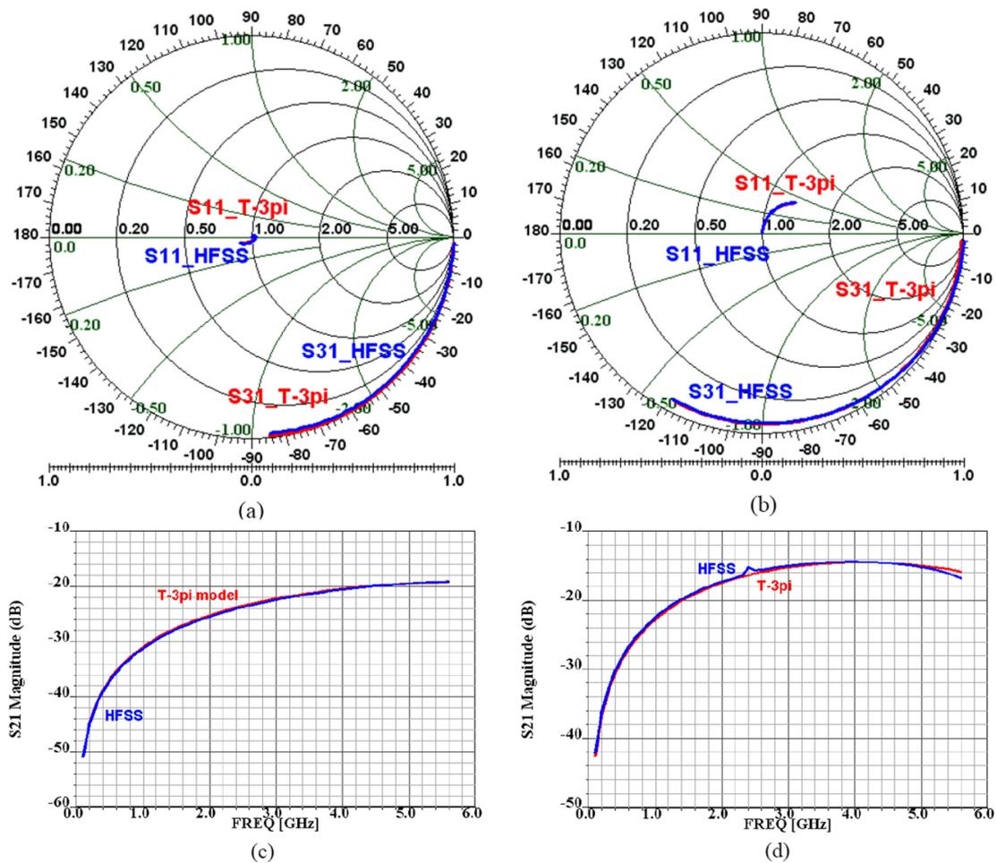
Fig. 10.  $S$ -Parameters generated from Ansoft HFSS and wideband T-3 $\pi$  equivalent circuit model. Data agrees up to 5.6 GHz. Smith chart of  $S_{11}$  and  $S_{31}$ . (a) COHS-LF package. (b) BGA package.  $S_{21}$  magnitude chart (c) COHS-LF package. (d) BGA package. (Color version available online at <http://ieeexplore.ieee.org>.)
