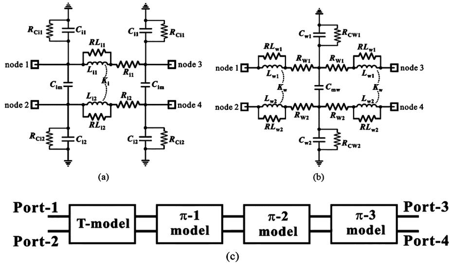
Fig. 9. Wideband equivalent circuit using T-3 $\pi$  model. (a) One section of  $\pi$ -model,  $i = 1, 2,$  and  $3$ . (b) T-model. (c) The T-3 $\pi$  model is consisted of a T-model in series with three cascaded  $\pi$ -models.
