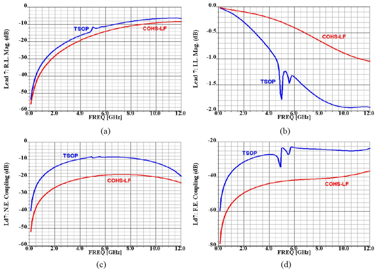
Fig. 6. Comparison of  $S$ -parameter in magnitude between COHS-LF and LOC-TSOP. (a) Return loss of Lead 7 ( $S_{11}$ ). (b) Insertion loss of Lead 7 ( $S_{31}$ ). (c) Near-end coupling of Lead 7 ( $S_{21}$ ). (d) Far-end coupling of Lead 7 ( $S_{41}$ ). (Color version available online at <http://ieeexplore.ieee.org>.)
