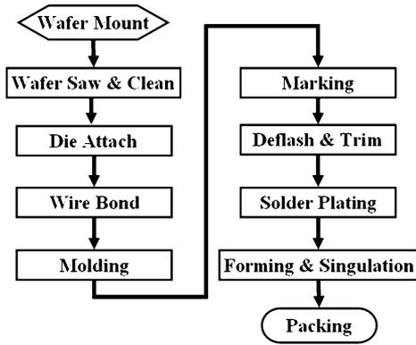
Fig. 2. Standard process flow of leadframe packages.
